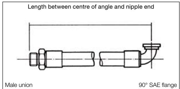
Remember that hydraulic hose under pressure will elongate up to 2% of its length or contract up to 4% depending on pressure, type and size. Sufficient allowance should be made to permit such changes in length.
