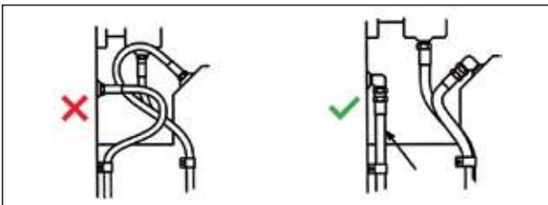
Obtain direct routing of hose through use of 45° and 90° adapters and fittings. Improve appearance by avoiding excessive hose length.
