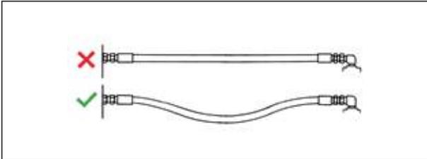
Since hose may change in length from +2% to -4% under the surge of high pressure, provide sufficient slack for expansion and contraction.
