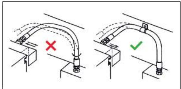
To avoid twisting in hose lines bent in two planes, clamp hose at change of plane, as shown.
