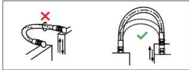
Never use a bending radius less than the minimum shown in the hose specification tables. Avoid sharp bend in hose to reduce collapsing of line and restriction of flow by using proper spring guard. Exceeding minimum bend radius will greatly reduce hose assembly life.
