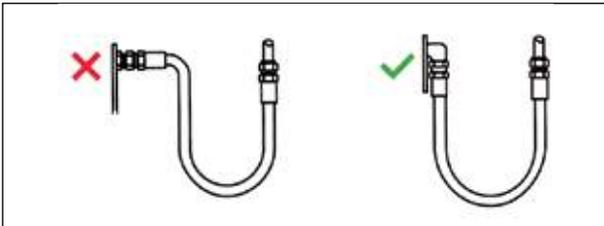
Avoid sharp twist or bend in hose by using proper angle adapters.
