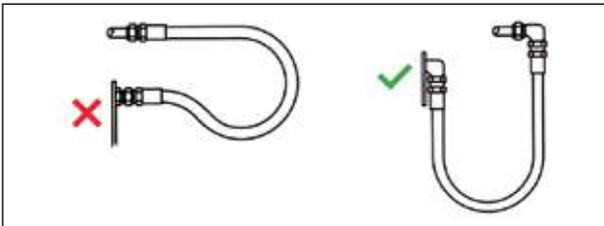
Where the radius falls below the required minimum, an angle adapter should be used as shown above to avoid sharp bends in hose.
