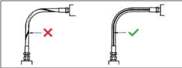
Hose should not be twisted. Hose is weakened when installed in twisted position. Also pressure in twisted hose tends to loosen fitting connections. Design so that machine motion produces bending rather than twisting.
