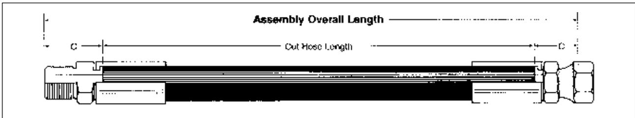
For most assemblies, the correct assembly length may be determined by direct measurement of the equipment or a drawing. Minimum bend radii as shown in the hose specification tables should be observed. Assemblies are measured to the end of the seal.
